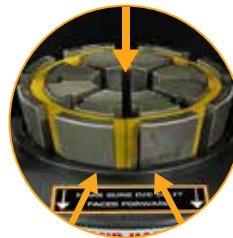
Crimp diameter is controlled by specific die and spacer combinations
