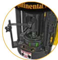
Coupling Stop makes repetitive crimps faster
