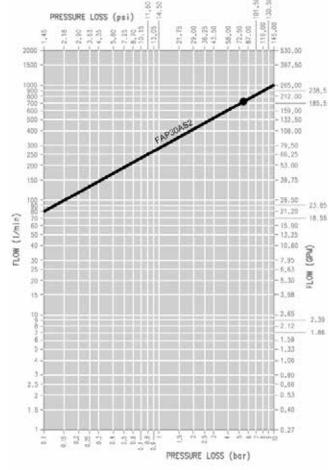
OIL = ISO VG32, TEMP = 40C, VISCOSITY = 28.8-35.2 MM<sup>2</sup>/S
